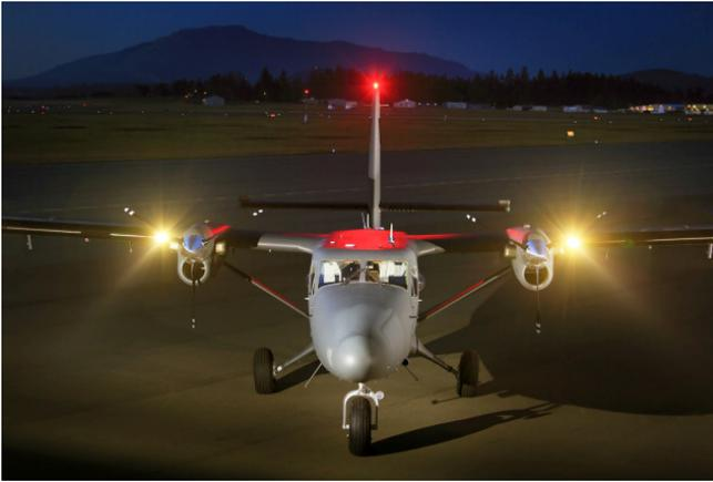
Pictured Above: The GAL Series 400 Twin Otters feature intermediate flotation gear (IFG) to facilitate operation on loose sand prevalent throughout the Arabian Gulf region.
